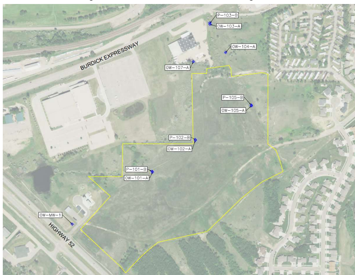
Figure 2.08b.1: Groundwater Monitoring Wells
