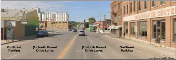
STREET-SECTION A-A EXISTING CONDITIONS
